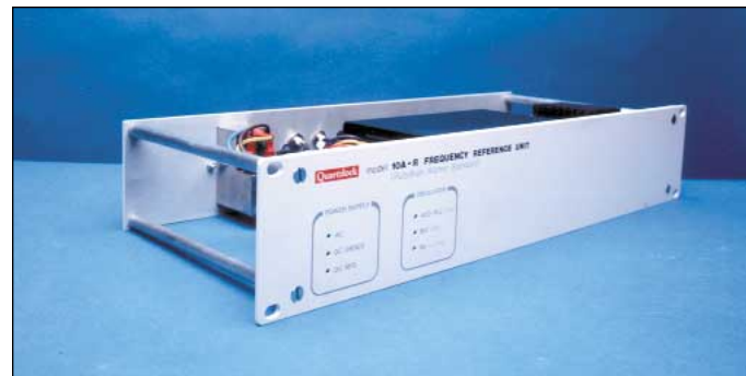
▲ Figure 4. A commercial rubidium standard.
